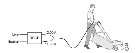
The RCCB would stop someone getting an electric shock from a faulty circuit in the lawnmower.
